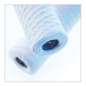
Honeycomb precision wound depth filter cartridges are manufactured to provide considerable dirt holding capacity, coupled with high flow rates and low pressure loss. Honeycomb elements consist of a metal or plastic perforated support core onto which yarn is wound at a pre-set rate, providing each rating of element with its own distinctive winding pattern and performance.
