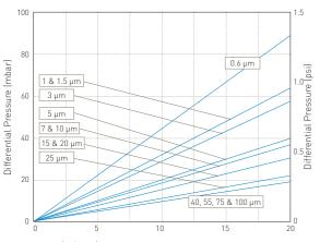
Flow (L / min) for liquid @ 20 °C and 1 cp per 10" module
