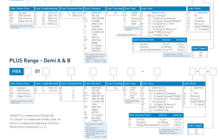
Note: All Tri-Clamp® connections conform to BS4825 Pt. 3
