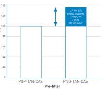
ODC technology combines fine particle retention with increased strength and stability to enhance the performance offered by the PREPOR range.
