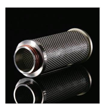
BIO-X II air sterilization filter cartridges utilize a borosilicate microfibre media. This media has proven to be particularly effective in the removal of sub-micron particles as small as 0.01 micron, therefore ensuring the removal of all microorganisms, including bacteria and viruses.
