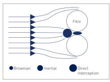
This is the dominant removal mechanism for the smallest particles captured by a filter in the gas phase Particles as small as 0.01 um exhibit great diffusional movement (Brownian Motion) which has the effect of increasing its nominal mean diameter to the filter. The efficiency of this capture mechanism decreases as the particle size increases.
